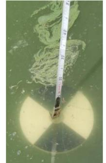
Secchi disk used to measure lake water transparency; algae scum sometimes on surface during calm conditions.
